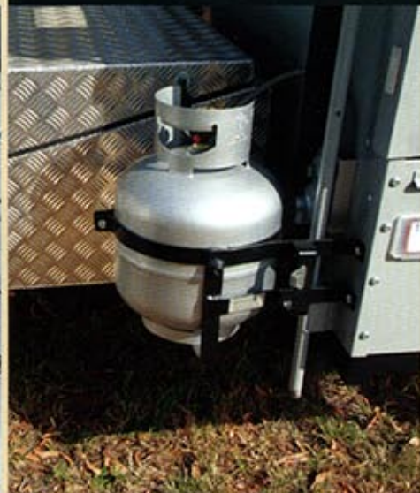
4 A 9kg gas bottle is tucked in behind alloy checker-plate stone deflectors
