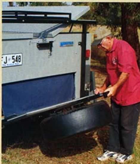
1 Drop the rear tyre and open up the tailgate
