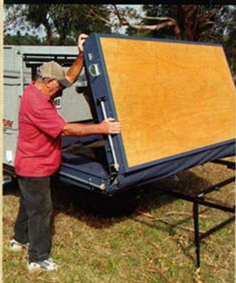
4 Open up the bed box to expose the tent canvas and its external frame
