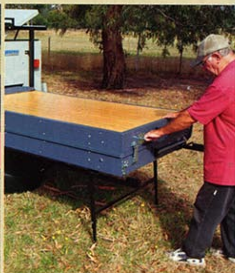
2 Slide out the bed base and extend the supporting legs
