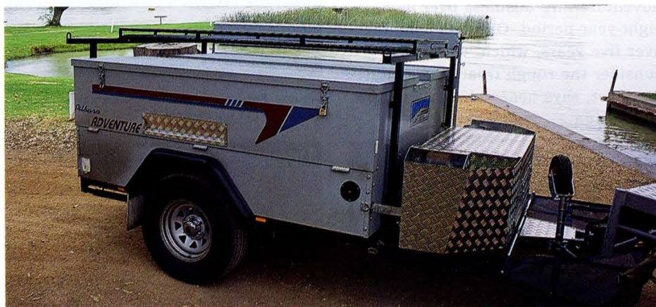
Below right: The spare tyre is mounted at the back of the unit and can be accessed even with a boat on the roof
